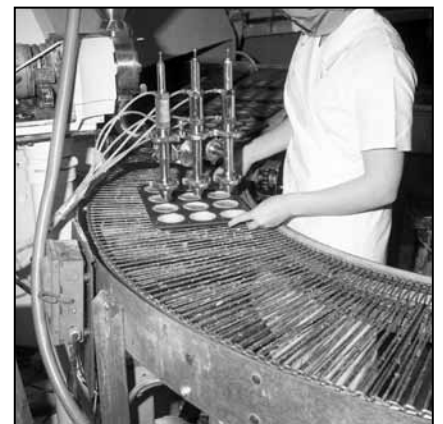
Production line at the new Flamingo Pastries plant on Simcoe St. (no Old Simcoe St.), in October 1968. Allan Rahm is seen with a fresh batch of dough, which will produce 500 dozen tarts. The stuffing of tart tins was still done manually, but the filling of the tart shells was done by machine.
