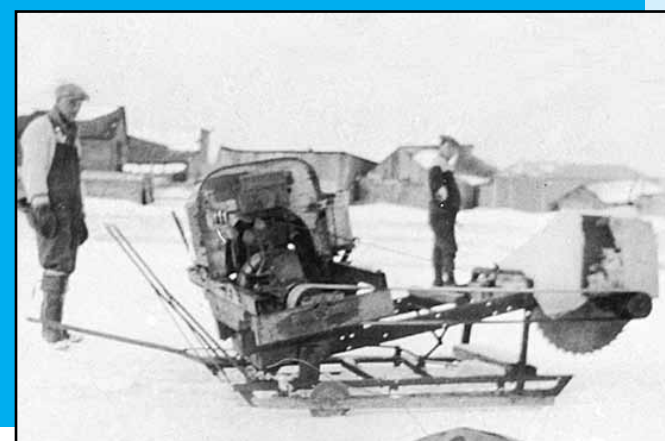
Men prepare to cut ice using this motor powered ice cutting machine on Lake Scugog about 1914.
