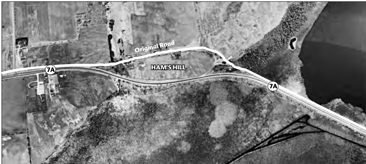
This aerial photo shows the original road to the Cartwright Causeway, (white outline) which had a very steep hill. In 1912 a new road was constructed at the bottom of Ham's Hill, to avoid the difficult and dangerous road. That road today is called Hwy. 7A.
