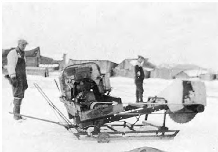
Men prepare to cut blocks of ice using this unique motor powered ice cutting machine on Lake Scugog about 1914.
