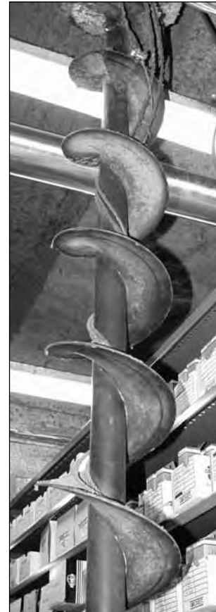
The grain auger, or screw conveyor, in the elevator.
