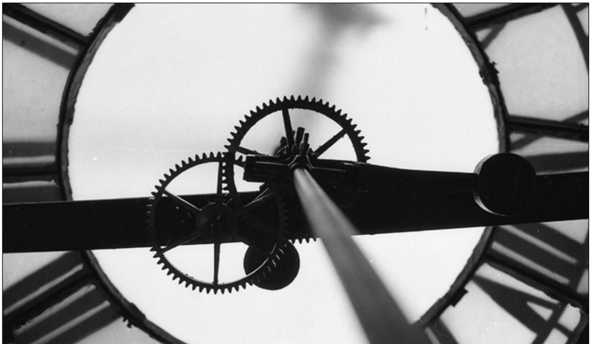
A long rod with brass gears attached to the face of the clock, turns the hands of the clock.
